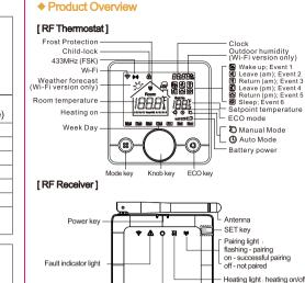
In this set, the thermostat compares the setpoint temperature with the room temperature, and decides if the receiver should switch the boiler on or off. And the receiver is wall-mounted and controls your boiler using existing wall-wires. With this set, you can regulate the room temperature everywhere you reach out.
